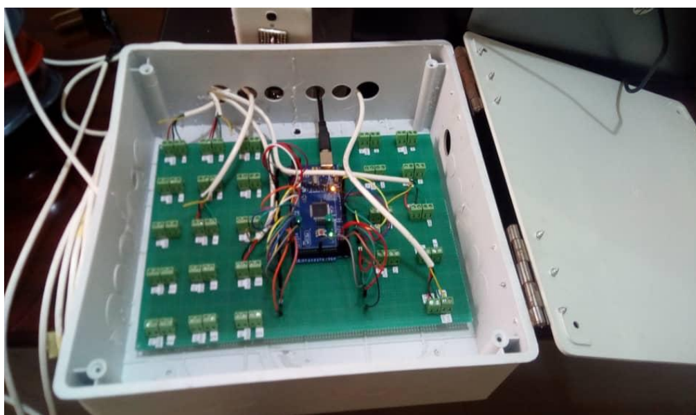
Fig. 5(b): The constructed low cost server-based automatic weather station with sensors connected
